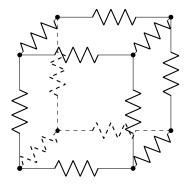
a) Assume that each edge is a resistance of  $2\Omega$ . If the +- and --poles of the battery are connected to the electric network as in below figure and the battery has a voltage of 12.6V, what is the total current from +-pole to --pole?
