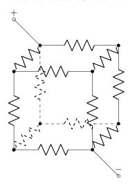
b) Assume that the situation is the same as in the previous part. An edge with a resistance of 5Ω is added to the electic network. The new edge is the diagonal of the cube connecting the vertex on the left-up-back of the cube with the vertex on the right-down-front of the cube. In other words: the new edge directly connect the poles of the battery, see below figure. By how much does the total current from +-pole to --pole increase by adding this edge?
